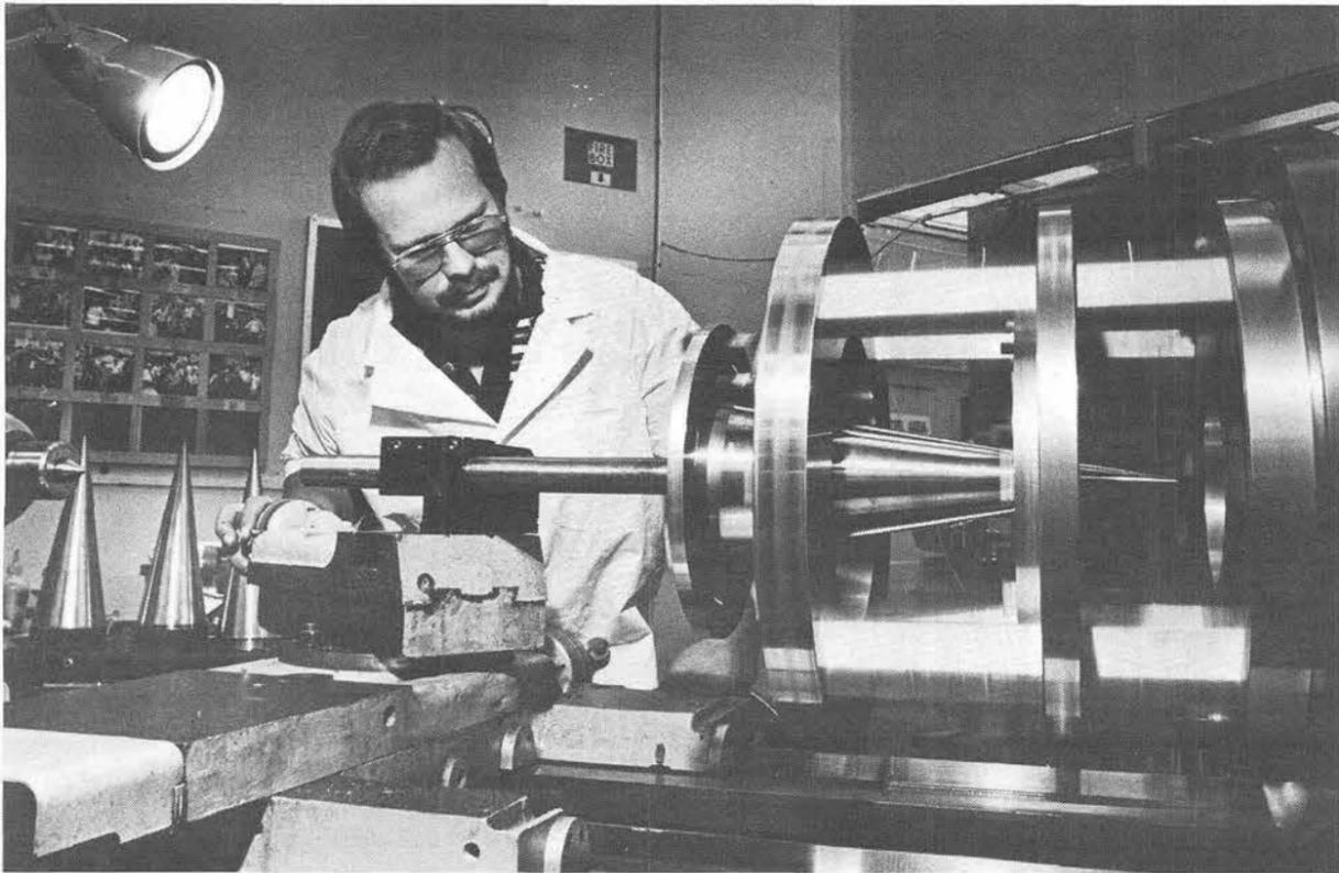
INSIDE a special holding jig, the nosecone of a rocket payload shapes up. Carl Brezowski, fourth-year machinist apprentice, makes an internal cut in the steel nosecone.
